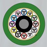
Duct FlexRibbon cables for FTTH applications
