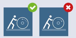
When rolling drums on the ground they shall be carefully "eased" over any rough surfaces and shall not be abruptly stopped by being rolled against a wall or other object. If a batten is damaged, it must be replaced immediately.
