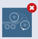
When using a fork-lift, the forks shall be long enough to support the full drum width. Always load the drum with the flanges perpendicular to the forks.
